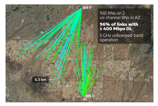
Multi-cell tests during G1's development demonstrated that its inter-cell interference cancellation was able to contain the capacity loss from k=1 deployment to less than 5% even in dense, conflicting conditions. The examples above show G1's inter-cell interference cancellation proven out in commercial deployment.
